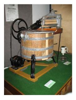
Rollers continued to be part of washing machines until the "spin" cycle was worked out after WWII. (The roller idea was patented in 1843. The first patent for an electric powered washing machine was issued around 1900.) Refinements in that period clearly took quite a while to be worked out, and were spurred on by other innovations (e.g. the electric motor) as well as gradual increases in household incomes.
